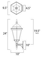
height from the center of outlet to the top of the fixture
