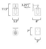
ight from center of outlet to the top of the fixture
