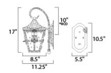
"height from center of outlet to the top of the foture
