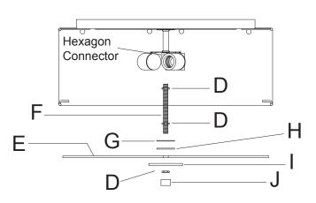
Thread the nipple into Hexagon connector, then secured by hex nut. Put the metal washer and rubber washer on the nipple, adjust them close to the glass diffuser by the hex nut, then put the glass diffuser on the shade spider, and put the Cap close to the glass diffuser, then secured by hex nut and finial.
