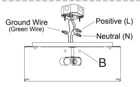
Wire fixture to wires in outlet box. Copper wire is for Ground. Attach canopy to mounting bracket and tighten with ball nuts  $_{\circ}$
