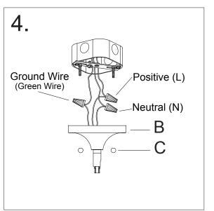
Wire fixture to wires in outlet box. Copper wire is for Ground. Attach canopy to mounting bracket and tighten with ball nuts.
