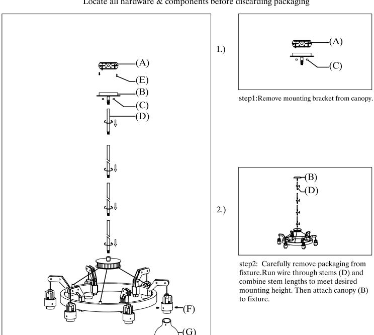
step2: Carefully remove packaging from fixture.Run wire through stems (D) and combine stem lengths to meet desired mounting height. Then attach canopy (B)
