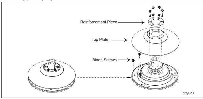
2. Assemble the fan blades to the motor assembly using the fan blade screws.(See Step 2.2)
