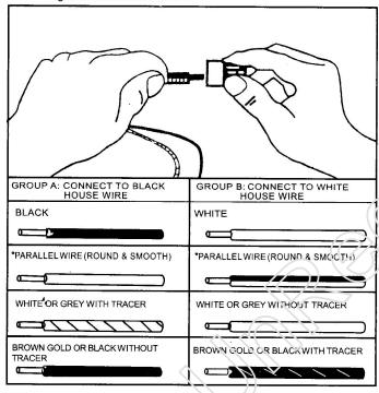
**NOTE:** When parallel wire is used, the tracer wire is square shaped or ridged, and the less tracer wire is round in shape or smooth. (Seen best when viewed from wire end.) To separate wires, grasp the ends of each wire and pull apart.
