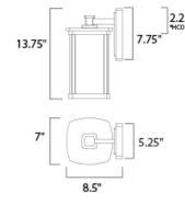
\*height from center of outlet to top of the foture
