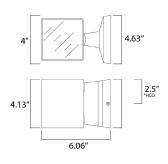
ight from center of outlet to the top of the fixture
